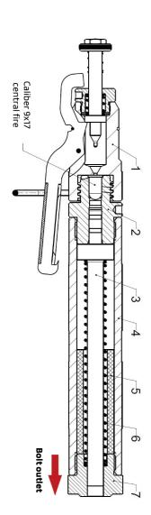
fig.: captive bolt stunner Blitz Kerner (loaded and tensioned)
